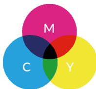
CMYK colors are subtractive. This means the starting point is a white canvas, and colors are added to block out parts of the color spectrum.
